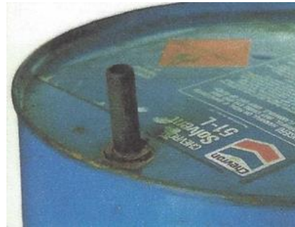
PLUGS NOT IN PLACE
