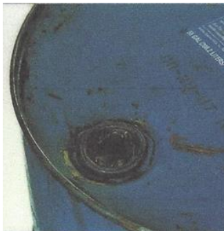
BUNGS OR PLUGS DAMAGED
